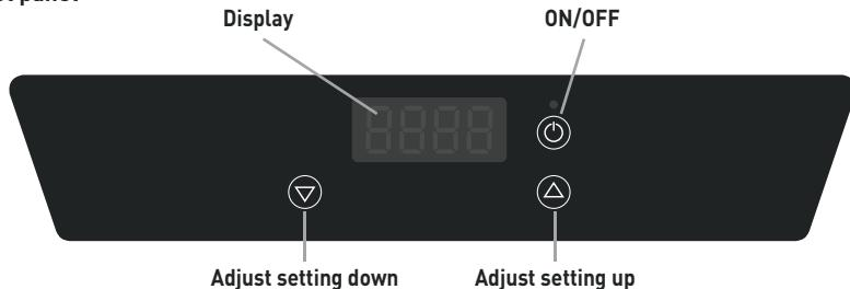
1. "ON/OFF" key: Use this key to switch the appliance on or to interrupt or reset the timer.
